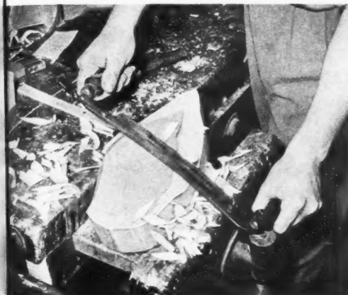
Assemble body sections with synthetic-resin glue, clamp until dry, remove clamps, and cut roughly to shape, employing a drawknife and a wood rasp.
